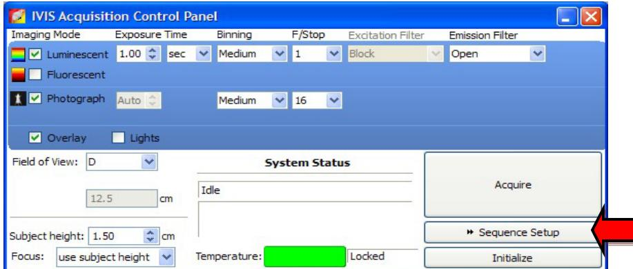
Enter values for exposure time, binning and f/stop and add to imaging sequence or select *Imaging Wizard* for assistance, set delay between images for a sequence with multiple images.
