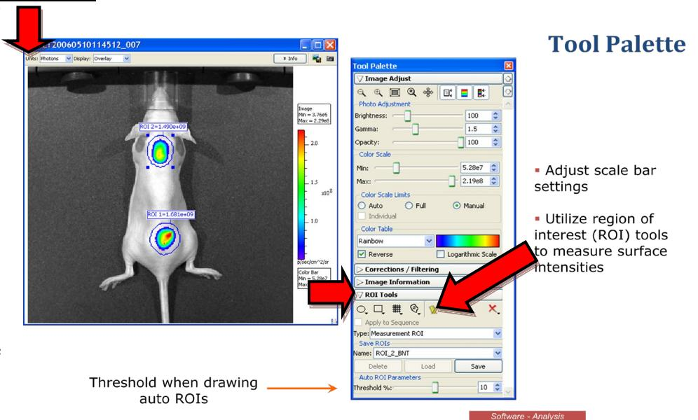
3. Measurement tool will display measurement of surface intensities within the ROI of each image.
