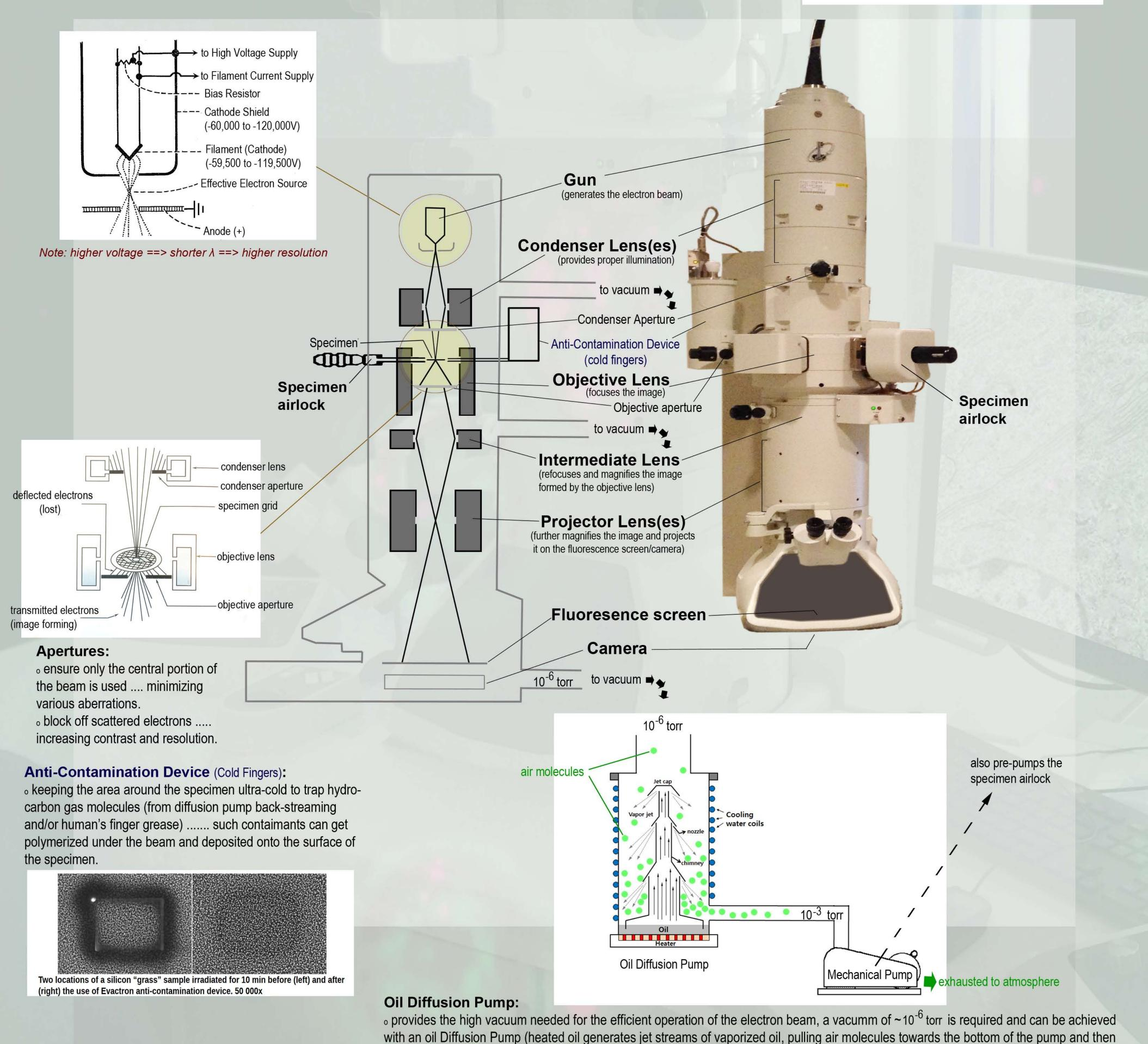
evacuated by a Mechanican pump; oil vapor condenses to oil on the cooled wall, draining back to the heater to repeat the cycle.
