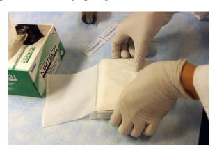
**Step 5:** Cut two pieces of cardboard the approximate size of the plate. Place the plate between the two pieces. This will help prevent damage during transport. Plates must be sandwiched between two pieces of cardboard prior to transport, not doing this may result in damage to the plates or seals.
