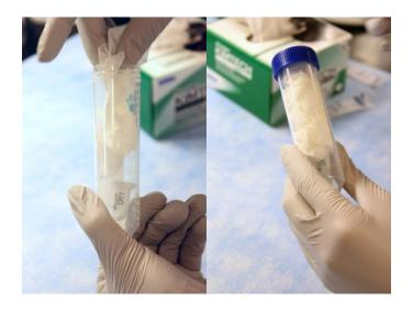
**Step 4:** Use parafilm to secure lid of the conical tube.
