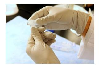
Step 3: Fill conical with samples and pack with kim wipes to ensure tubes do not shift during transit.
