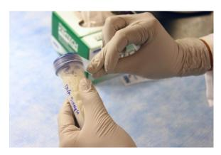
**Step 5:** Place conical in a clean plastic bag.
