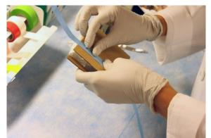
Step 7: Each plate must be secured in its own cardboard sandwich and sealed in individual bags.
