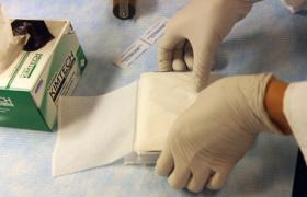
**Step 5:** Cut two pieces of cardboard the approximate size of the plate. Place the plate between the two pieces. This will help prevent damage during transport. Plates must be sandwiched between two pieces of cardboard prior to transport, not doing this may result in damage to the plates or seals.
