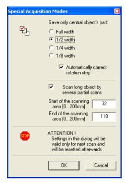
Save only central part option allow acquiring projection images for reconstruction of specific central part of the object, which can be 1/2, 1/4, 1/8 of the selected scanning width. It can reduce necessary disk space for scanning of small objects located in the central part of the specimen bed. Use "Object size > field of view" during reconstruction to avoid influence of the object bed and surrounded specimen parts.
