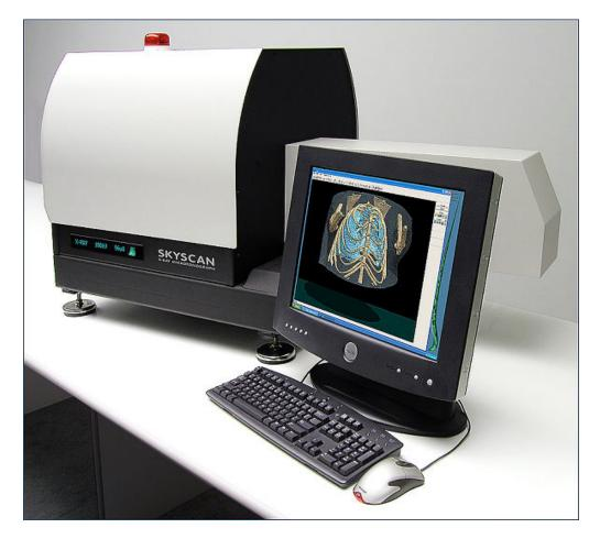
The equipment contains an X-ray microfocus tube with high-voltage power supply, a rotation stage with overall accuracy of <10 $\mu$ m, a translation stage, a two-dimensional X-ray CCD-camera connected to the frame-grabber and a Dual Intel Xeon computer with LCD monitor.
