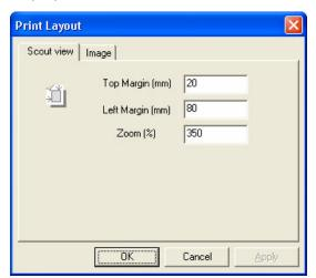
Print layout for scout view contains adjustments for printing position (margins) on the page and image scale as a zoom from original (corresponding to object size) format.
