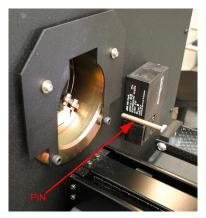
Remove the visual camera by pressing on the two sides of the fastening mechanism. Be careful that you don't damage the flat cable.
