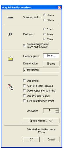
Scanning width should correspond to the size of scanning area (diameter of object bed). Sometimes possible to scan the central part of the big size object with small Scan width (central part will be scanned) -> Use "Object size > Field of view" option in the reconstruction program in this case.
