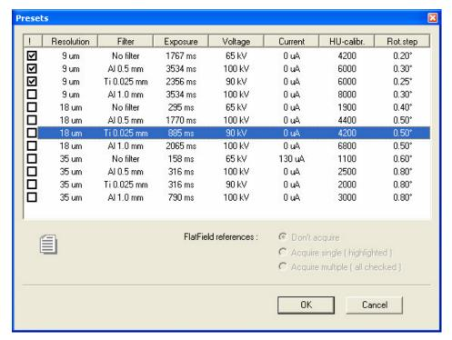
Top part of the dialog window contains a table with 12 acquisition modes for 4 available filters and 3 possible pixel sizes. For sorting according to specific parameter click twice to the corresponding column title.
