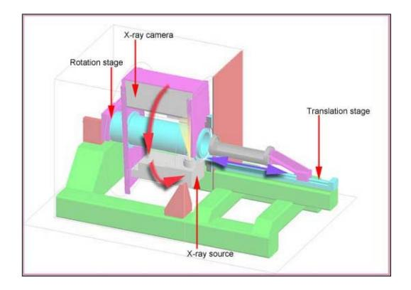
For "SkyScan-1076" the X-ray microfocus tube with 5 micron focal spot size operates at 20-100kV / 0-250 $\mu$ A. The special X-ray CCD-camera is based on 10 Megapixel (4000x2300 pixels) cooled CCD-sensor with fibre optic coupling to x-ray scintillator
