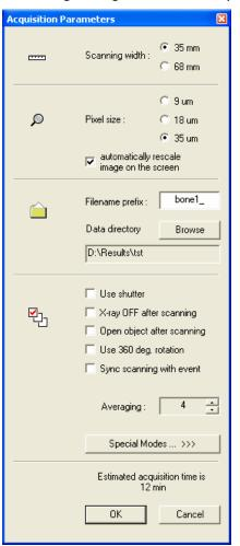
**Scanning width** should correspond to the size of scanning area (diameter of object bed).
