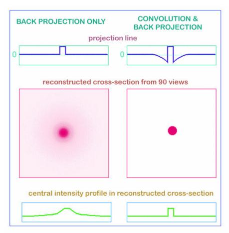
The same algorithm can produce the cross-section image not only from the single point object. Any real object can be represented as a big number of separate absorption voxels and linear absorption in any x-ray beam is corresponding to the sum of all absorption from all voxels inside this beam. By this way the two-dimensional cross-sections of the object can be reconstructed from the one-dimensional shadow lines in different views.
