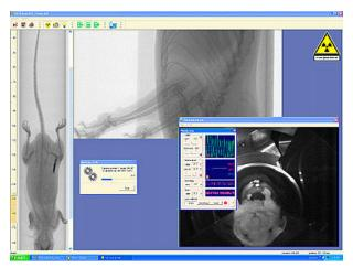
Left part: scout view (up to 200mm) with selection of the scanning position. Central part: real-time x-ray image and progress indicator; Right bottom part: physiological monitoring and real-time visual image of the animal.
