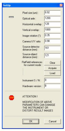
**Pixel size** adjusts the size of the image pixel in the object plane for the maximum camera resolution.
