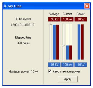
Left part of the dialog box shows information about the type of x-ray source, elapsed time (active emission) and maximum available power.
