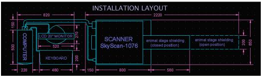
The table, on which the system will be put, should be strong enough to support a weight of 150 – 200 kg. The distance between the backside of the system and the wall should be at least 10 cm, necessary for the airflow.
