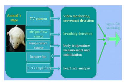
The TV-camera in the animal bed produces real-time visual image. Operator can see the animal on the computer screen in any time including x-ray scanning. Special software detects local movement of the animal body. This information can be used for scanning synchronization with animal's breathing.
