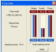
Left part of the dialog box shows information about the type of x-ray source, elapsed time (active emission) and maximum available power. Right part is used for indication of current values (red) and adjustment for new values (blue). New values can be applied by pressing to Apply button. The voltage reaches from 0 to 100 KV, the current from 0 to 250  $\mu$ A.
