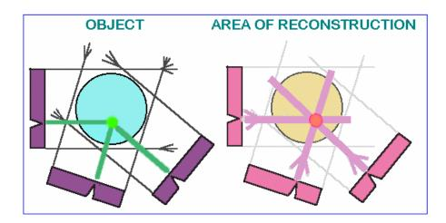
Now let's rotate our object and repeat this operation. In each new rotation position of the object, we will add to the area of reconstruction the lines of possible object positions corresponding to position of shadow. This operation is named "back-projection". After several rotations we can localise the position of the absorption point inside the area of reconstruction. In increasing the number of shadow projections from different views this localisation become more and more defined.
