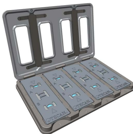
Figure 103: Cell chip adapter with springs (dark gray)
