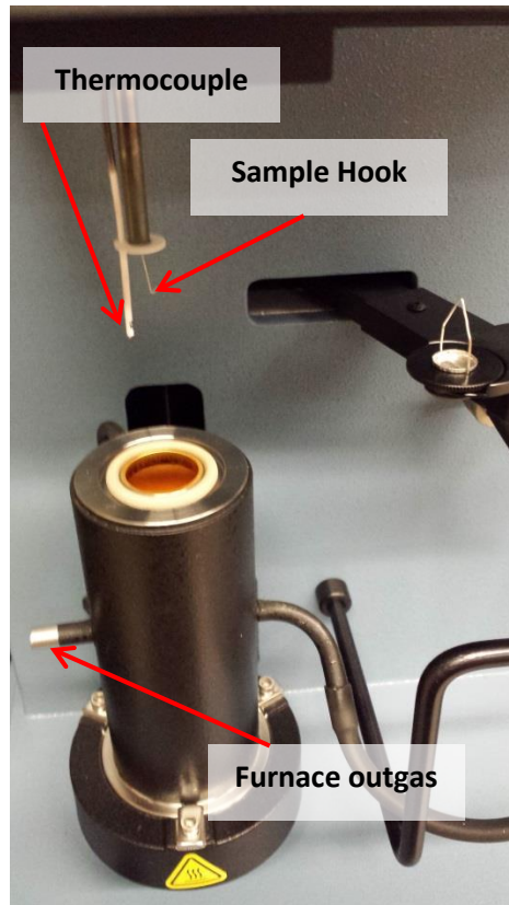
Fig. 5, a close up of the furnace. The thermocouple should be very close to your sample but not in any danger of being touched by your sample when it undergoes thermal expansion.
