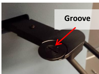
Fig. 3 , shows the groove in the autoloader arm. You need to line the sample pan wire up with the groove until it is in place. The autoloading function will not work if you do not do this.
