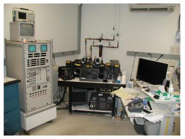
The MoFlo Legacy can simultaneously analyze and sort up to 6 different colors by choosing different detection filters. The filters and detectors can be easily reconfigured and exchanged for color detections based on the experimental design. It has been in service since 2001. It still functions like new.
