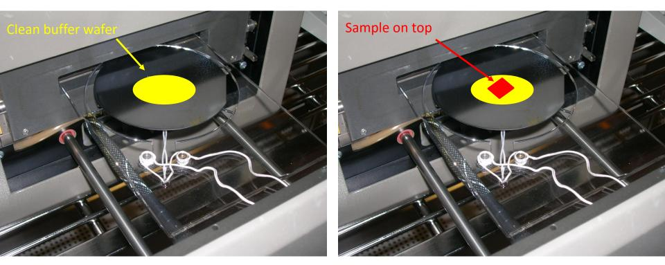
\*\* This prevents contamination from the chuck to your sample! \*\* Buffer Wafer should be any piece of silicon cleaned in Piranha for 10 minutes \*\* DO NOT move or handle the thermocouple wafer – it is very fragile
