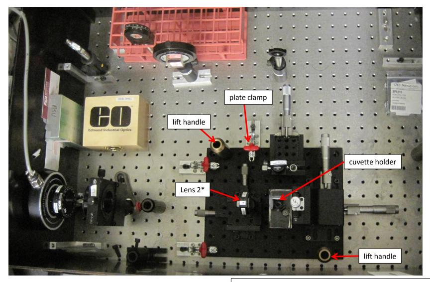
\* Lens 2 is shared with base plate for liquid based measurements. Orient lens with arrow pointing towards detector.
