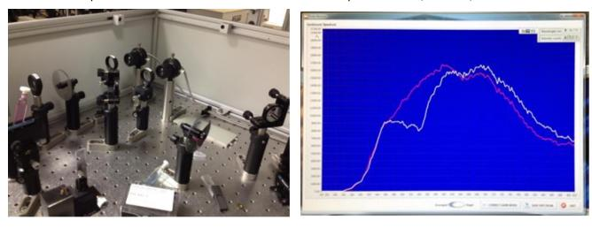
12. **Align pump and probe beams** place alignment tool in sample holder and let the probe beam through the pinhole; adjust pump beam through the pinhole using the mirror with BLUE knobs. There are 2 pieces of alignment tools; the black one has a smaller pinhole (!!keep both of them in the EOS box). Replace the alignment tool with sample, maximize the signal in 'ADJUST OVERLAP' window with appropriate time delay
