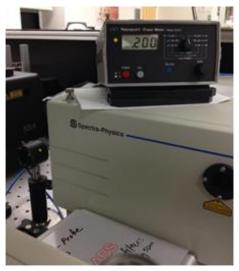
6. **Align excitation beam** use the mirror at OPA exit to guide beam to the first iris; using the 2 folding mirrors to direct the beam through the second iris and the EOS entrance; place a card in EOS to monitor the beam
