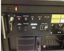
10. **Set probe light** in EOS program, open 'MONITOR PROBE' page; slowly turn the 'POWER KNOB' while monitoring the number in the 'POWER SETPOINT' window, and the spectra (white=probe, red=reference) in the 'MONITOR PROBE' page on screen. !! Keep laser power below 0.860 to prevent laser damage!!
