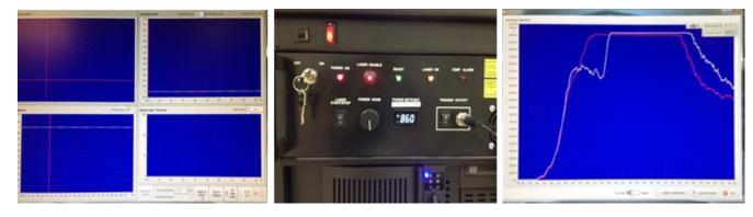
11. adjust probe and reference beam intensities detectors saturate at  $\sim$ 20,000 counts, use 3 NG filters to balance the probe and reference beam intensities and to keep both at  $\sim$  18,000 – 19,000 levels
