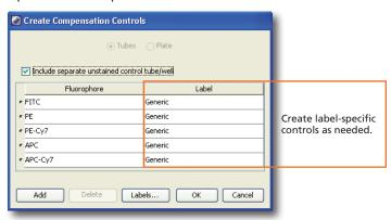
4 Install the unstained control onto the cytometer. Click Acquire Data.
