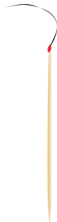
Fig. 7. Sectioning tissue for EM: Collection supplies. Eyelash brush made for collecting thin sections (Subheading 3.6, step 7).
