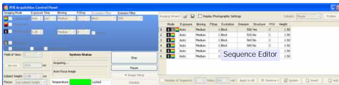
Figure 4.17 Control panel and sequence editor during acquisition Each row in the sequence editor specifies the acquisition parameters for one image in the sequence. For more details on the sequence editor, see Table 4.5, page 40 .
