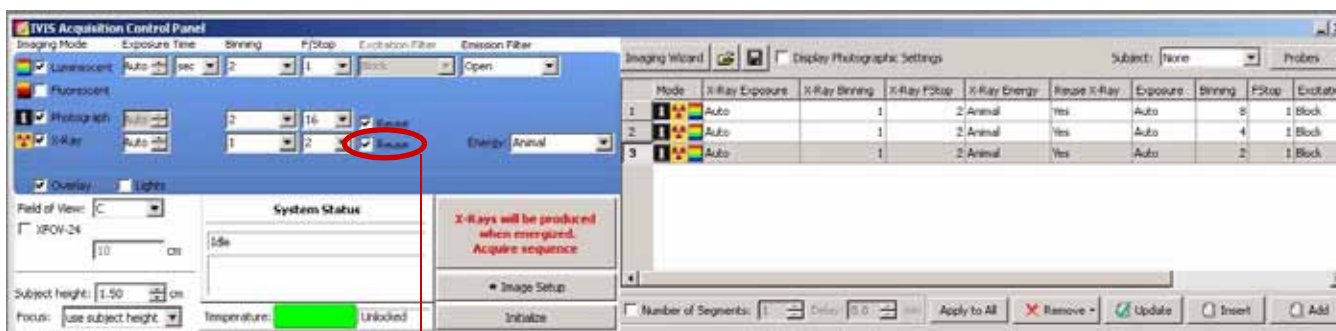
X-ray reuse option is selected by default. One X-ray image is acquired for the sequence.
