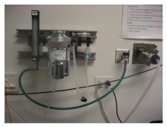
Oxygen to all wall mounted units is turned on at the wall (black tap). Some units have an additional flow controller upstream of the vaporizer unit (as shown left), and some systems have additional flow controllers downstream of the vaporizer to allow control of flow to different outlets (such as induction chambers and imaging instruments, and shown on the bench-top unit image below).
