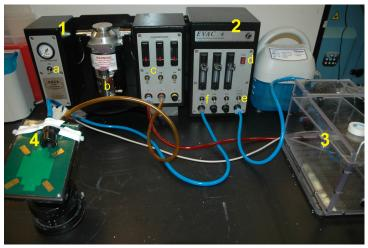
The new SAS3-EVAC4 systems allow controlled isoflurane delivery and scavenging for up to three outlets. The SAS3 unit (1, right) has a switch on the left side of the unit (a) that will pressurize the entire unit to ~6psi, and three flow controllers (c) to the right of the vaporizer (b) to deliver anesthetic gas to the induction chamber (red outlet) and two other outlets (orange and yellow). Note that the flow to each of these outlets is preset. The EVAC4 pump (2) is turned on
