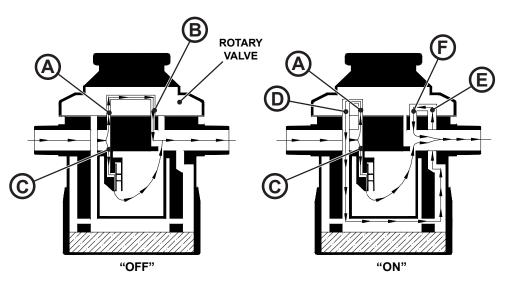
Figure 2 Schematic – Principle of Operation
