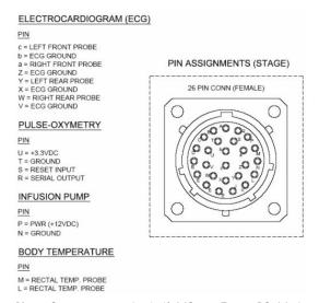
**Note:** Connector type in shelf–MS3119E16-26PS. Mating connector required (supplied by customer). Manufacturer: Amphenol Aerospace, part no. MS3126F16-26P.
