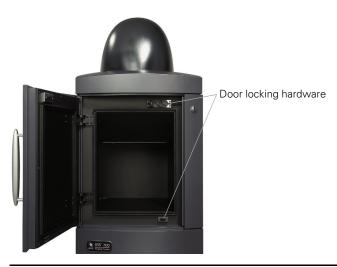
Figure 6.3 IVIS® Spectrum, imaging chamber
