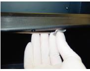
The stage lock down bar is located at the bottom front edge of the imaging platform.
