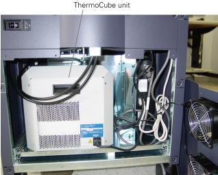
Figure 10.2 Removing the lower rear panel using a hex head wrench (left) and ThermoCube unit exposed (right)
