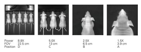
Figure 6.4 Example field of view obtained with different lens configurations
