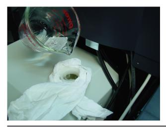
Figure 10.5 Adding coolant to the ThermoCube unit
