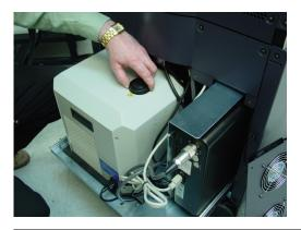
Figure 10.4 Removing the fill cap
