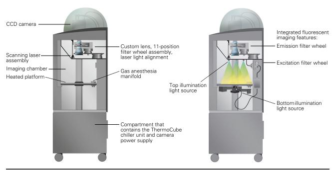
Figure 6.1 IVIS Spectrum components
