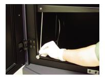
Pull the bar down from the stowed position and place it as shown above. Return the bar to its stow position before returning the imaging platform to the operating position.
