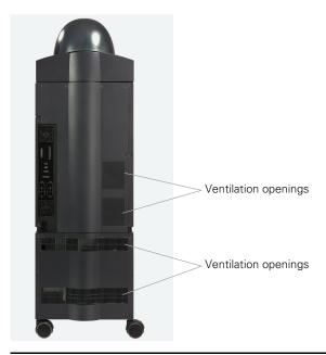
Figure 6.7 IVIS Spectrum, back view
