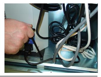
Figure 10.3 Loosen the tray locking bolt
