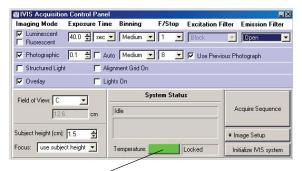
The temperature square is red at startup and turns green when the operating temperature is reached. Click the temperature square to display the demand and measured temperature of the CCD and stage.
