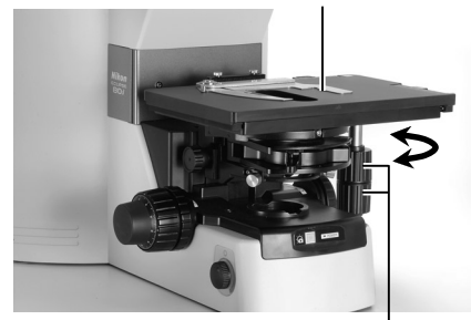
Move the portion to be viewed into the optical path using the XY stage knobs.
